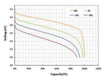
CHARGE : CC(0.5C)/CV(4.2V to 0.1C) at 25°C DISCHARGE : CC(0.5C) to 3.0V at various temperature
