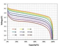
CHARGE : CC(0.5 C)/CV(4.2V to 0.1C) at 25 °C DISCHARGE : CC to 2.7V at 25 °C
